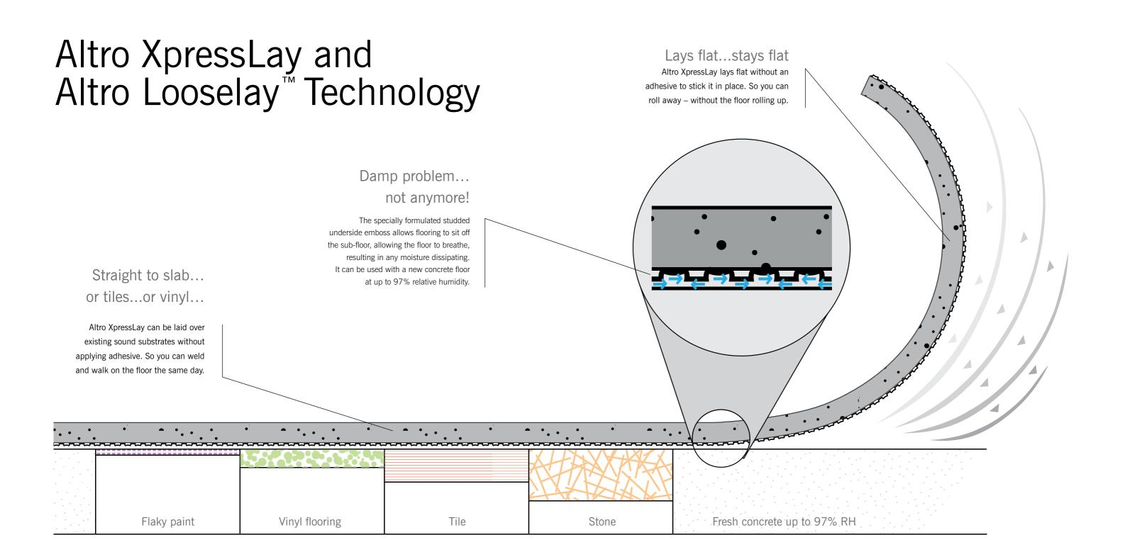
Altro XpressLay utilises Altro Looselay Technology for a quick fit without compromising on safety or durability.
